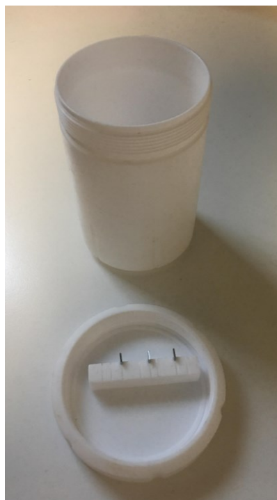
Figure 2-1: Photograph of the Teflon™ container and sample holder used in the water treatment as well as in the hydrogen peroxide treatment.
