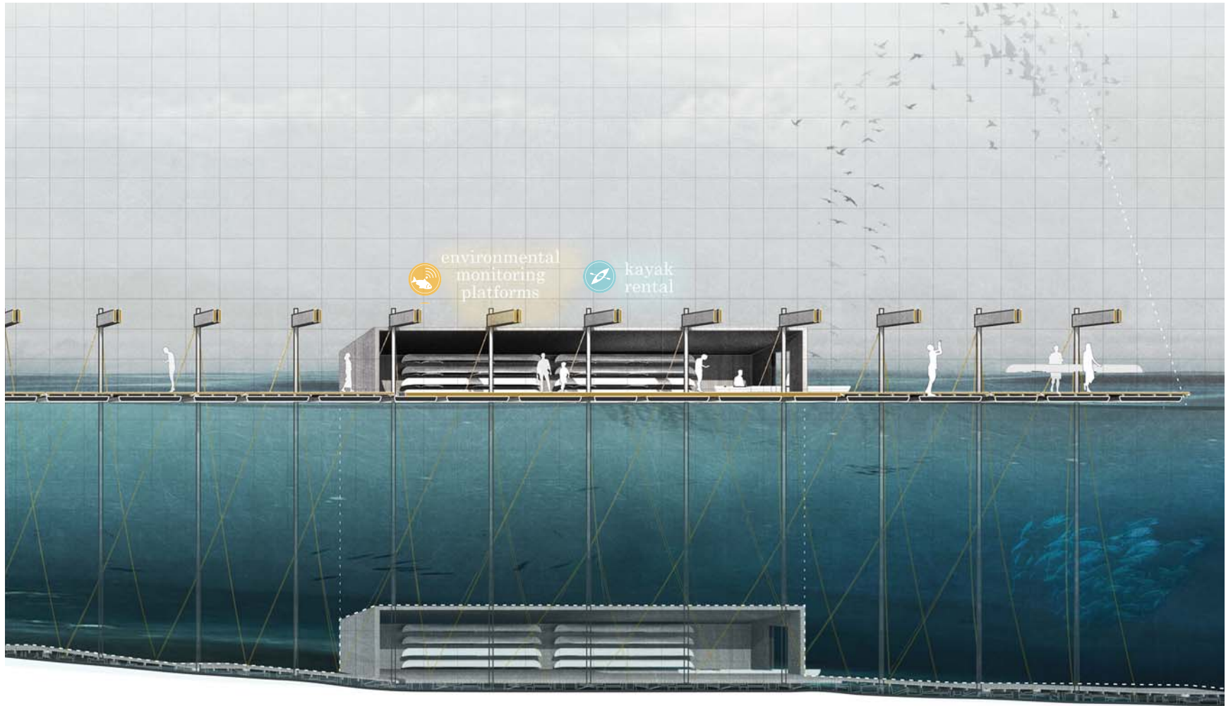
Closer view of the inhabited boat bridge section shown at high tide, with the low tide position ghosted in. The boat shed houses kayaks and environmental monitoring equipment, combining energy and community program related to the tides.
