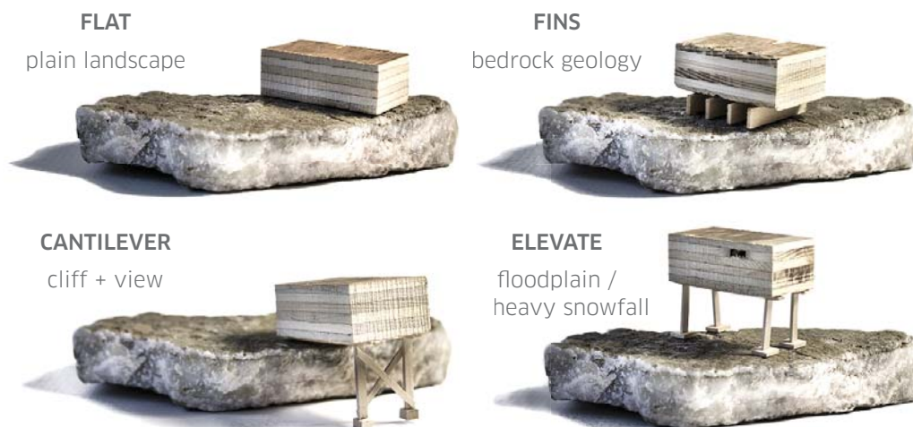
Early sketch models demonstrating ways structure may adapt to various landscape conditions.
