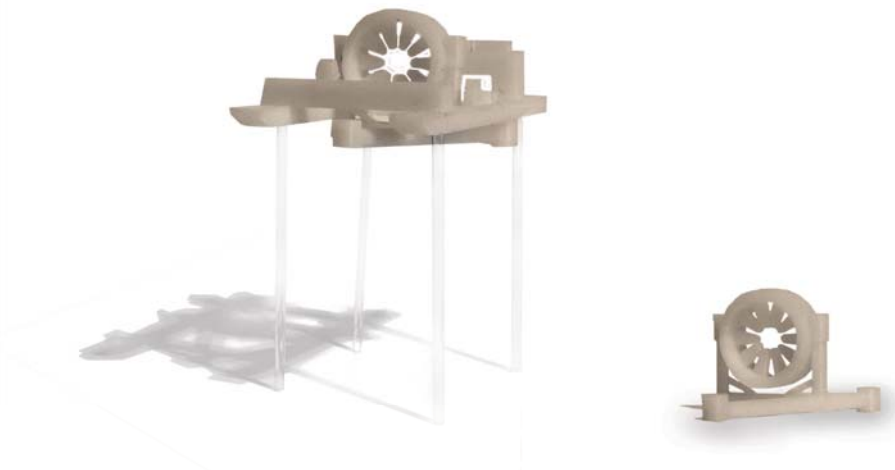
Physical model of the OpenHydro turbine. Left: The turbine shown at the waters surface, 45 metres above the ocean floor, secured in the Scotia Tide Barge, a device that was designed and built specifically for installing this large turbine. Right: The turbine as it sits on the ocean floor.
