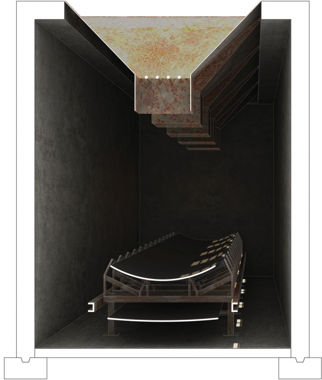
Figure 42: Existing conveyor tunnel with hoppers.
