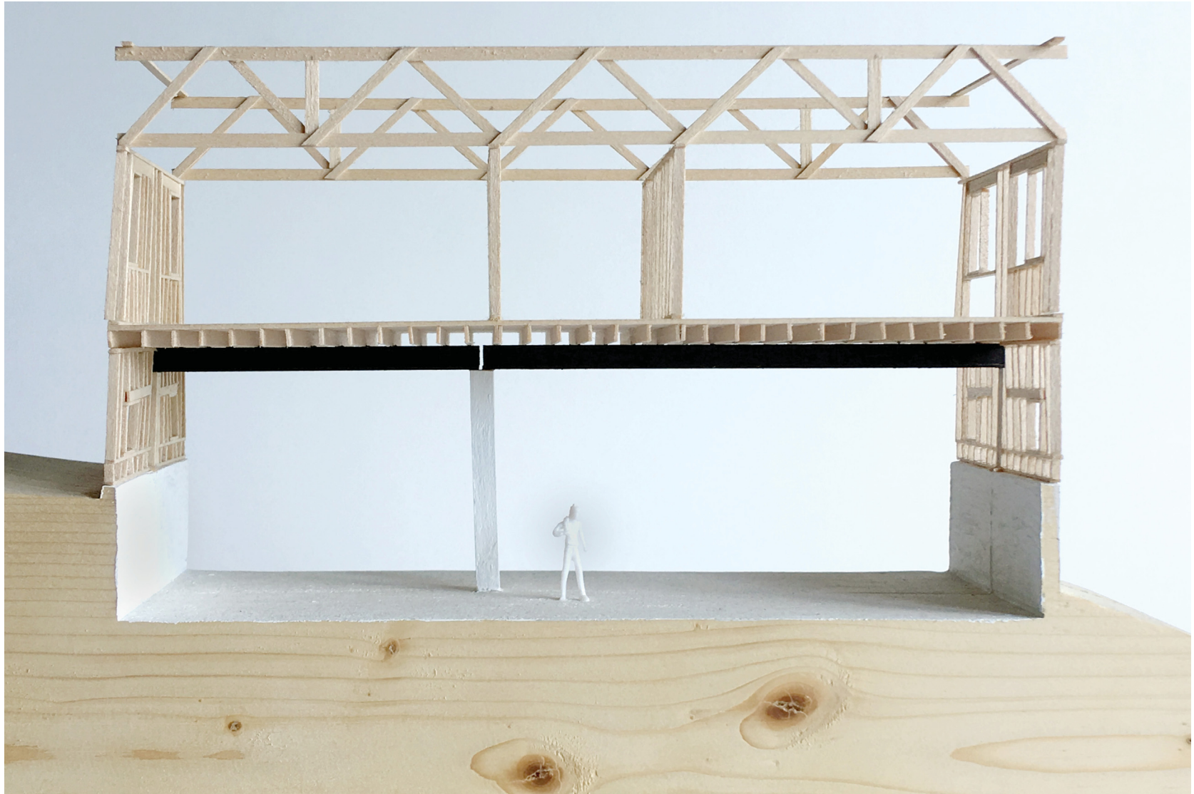
Fig.93 Study section model to understand the building's construction. The white represents concrete; the black represents steel beams.
