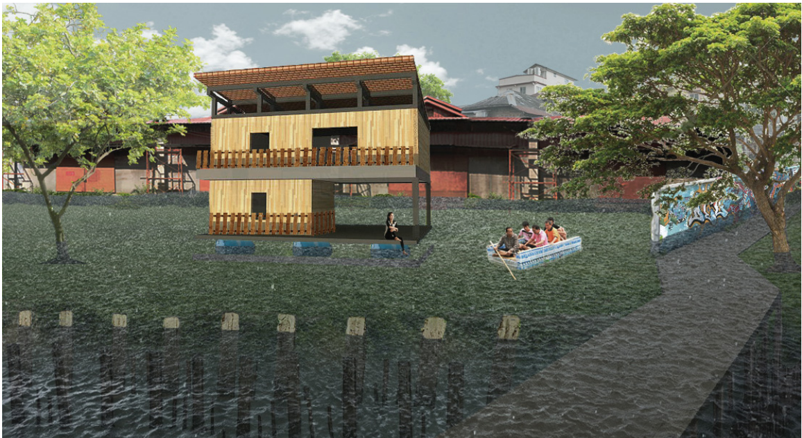
Rendering of how a structure can be retrofitted to be amphibious and float up within the concrete foundation to respond to flood events during the wet season.
