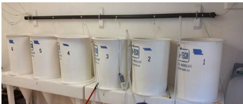
Figure. 9. Larval tanks (100 litres) used for rearing until pediveliger stage (pre-settlement) was achieved. Samples were shipped within 24 hours to VIMS for flow cytometry
