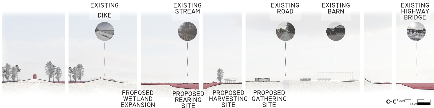
Section C-C' proposed landscape section details showing the relationship between the rearing, harvesting, and gathering bio-habitats, the highway, the dike, and the stream. Images from Google Street View.
