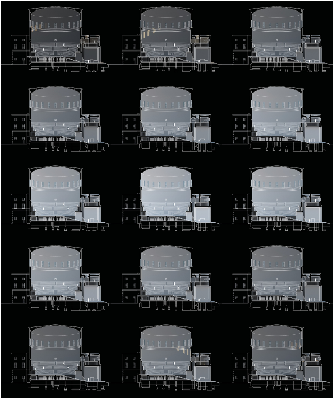
Figure 29: Examining the Stockholm Public Library by Erik Gunnar Asplund built in Stockholm, 1928 and located at 59.3^{\circ} N. Base section from Erik Gunnar Asplund, Public Library, MoMA Archive. Study uses the 3D modelling software Rhinoceros and the rendering software V-Ray to simulate light over the course of one day, August 15, 2016, the day I visited.
