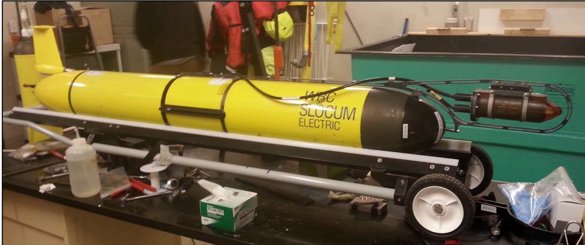
Figure 4. A Slocum Ocean Glider fitted with a Passive Acoustic Monitoring system (forward of the glider nose) used for detecting and identifying right, humpback, sei and fin whales in real-time.
