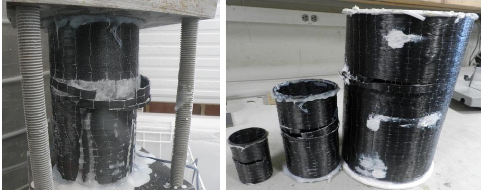
Figure 3. Typical ruptured FRP jackets
