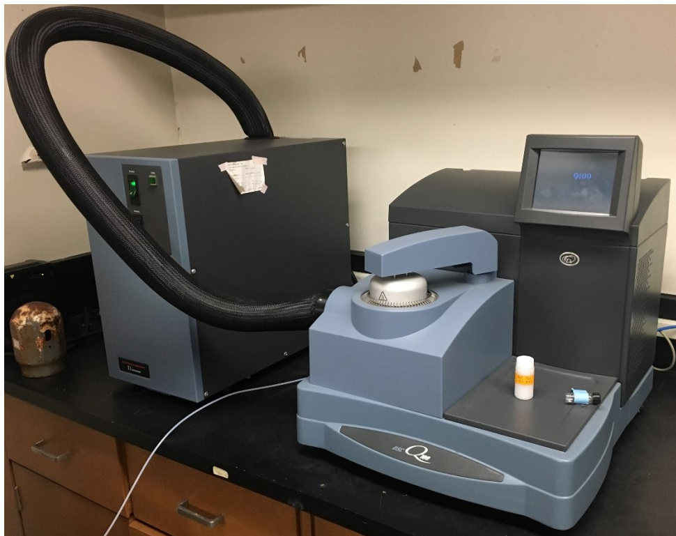
Figure 3.2 TA Instruments heat flux DSC Q100 equipped with modulated DSC connected to a refrigerated cooling system, RCS.
