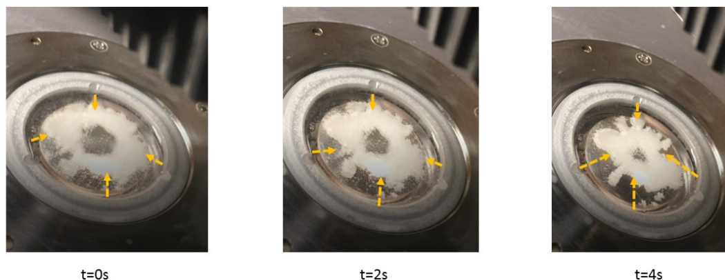
Figure 4.17 The movement of SSS molecules on the quartz plate on the bottom plate
