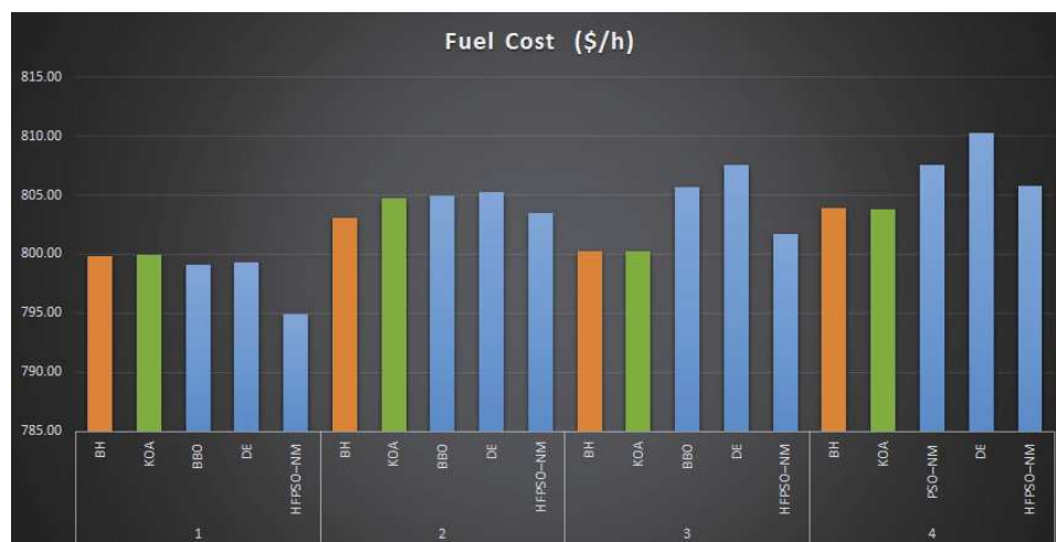
Figure 10.7: Comparison of BH and KOA optimization algorithms fuel cost results with other algorithms in literature without wind energy and the load reduction is not active
