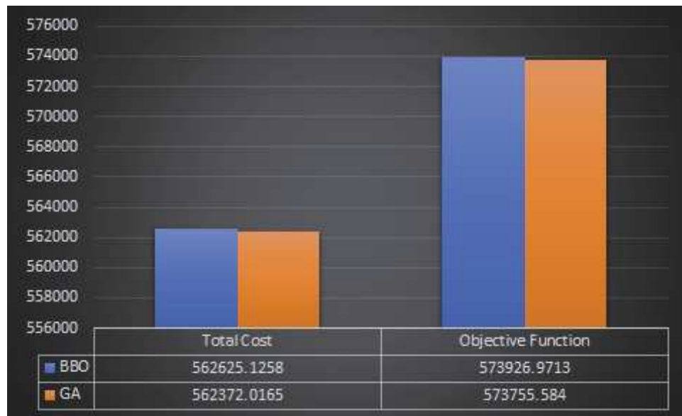
Figure 8.7: Optimal results of ten thermal generation units without wind energy and the load reduction measures are active at peak loads for twenty-four periods of time and the spinning reserve on the thermal units is assumed to be 10% of the demand at each period
