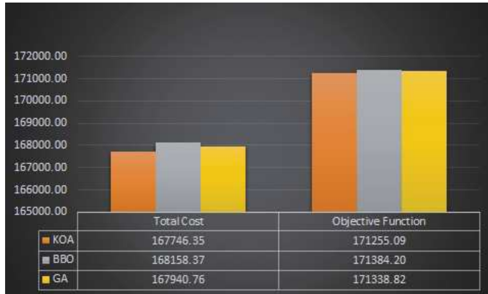
Figure 9.2: BBO, GA and KOA algorithms results of test system 1 with wind energy and load reduction is not active
