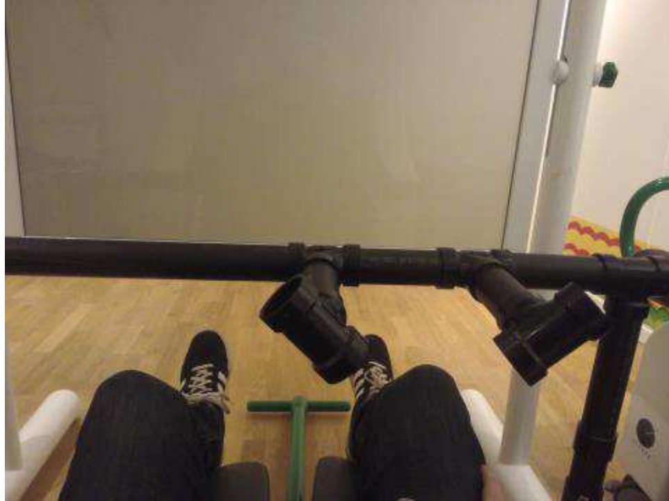
Figure 10: Experimental apparatus used. Two targets (rotated 45° and 135° above the horizontal) were presented to the participant on either side of their right leg.
