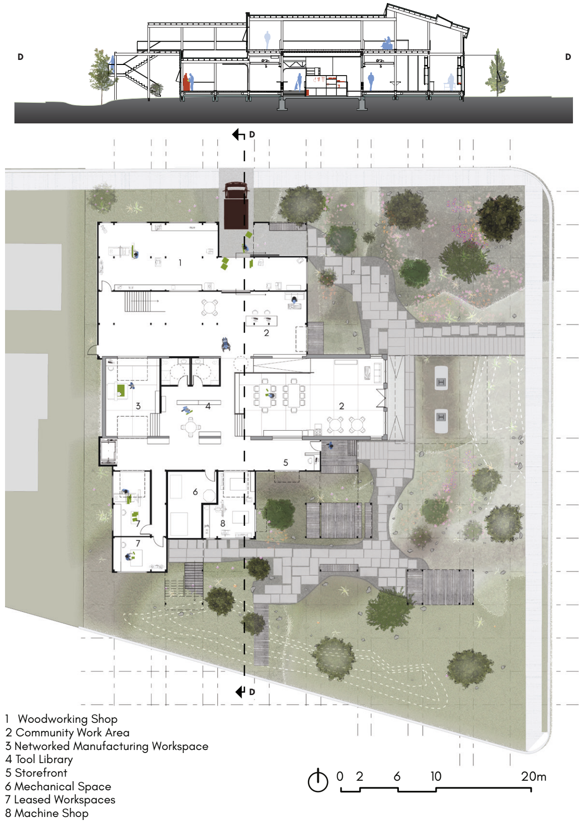
Figure 47. Projected plan, with accompanying section, of the building and landscape twelve years after the initial occupation.
