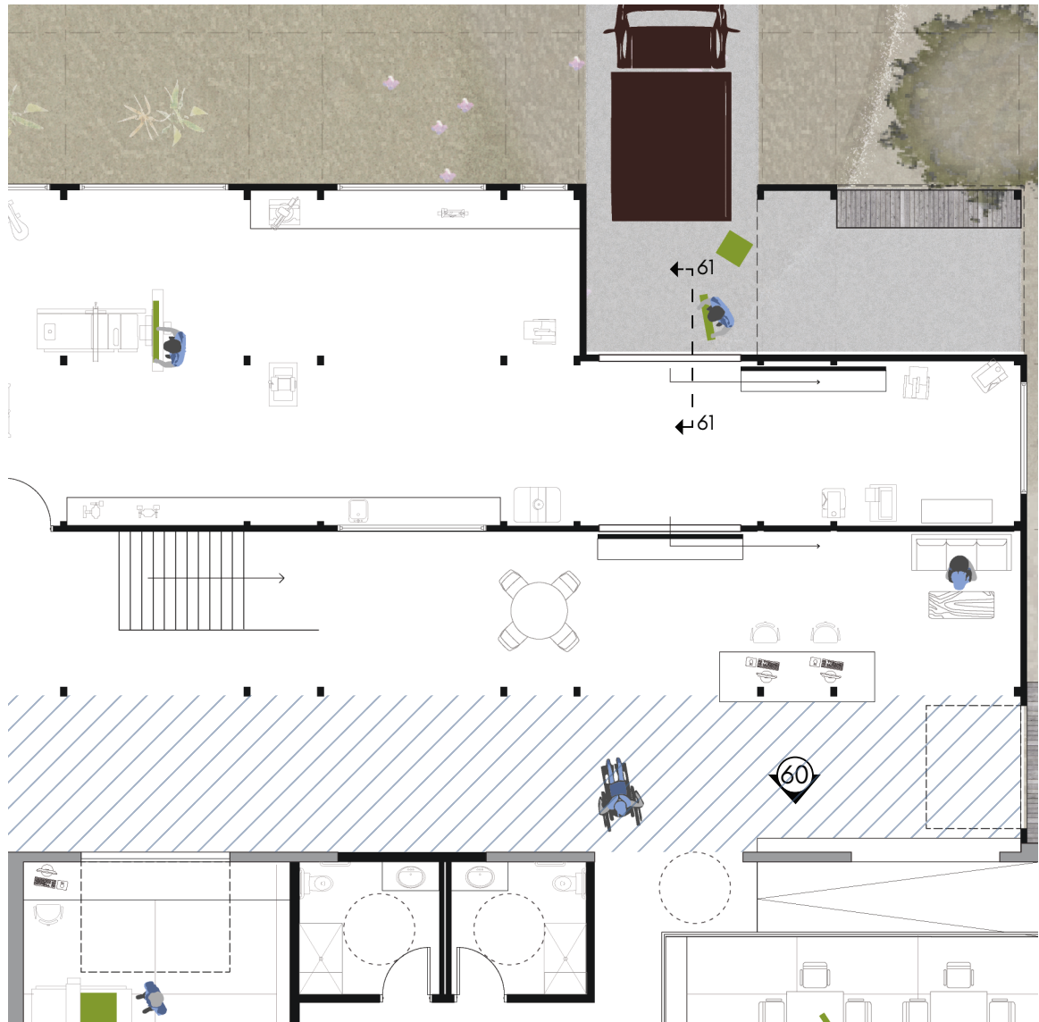
Figure 58. Key plan of workshop space. Spaces immediately adjacent to the existing building (hatched) become dedicated circulation space that can also be part of larger social or work spaces.
