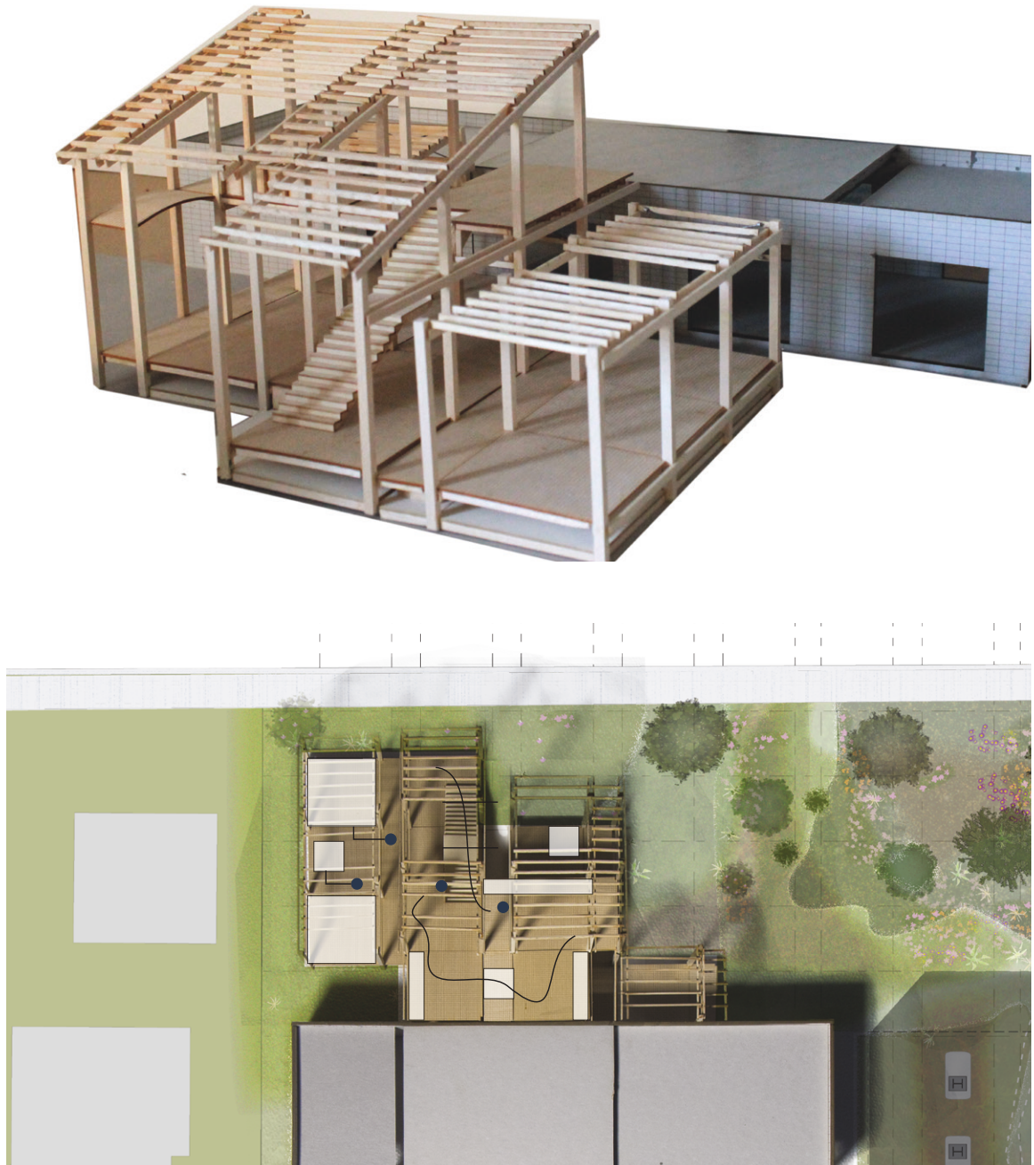
Figure 53. This workshop scheme, based on timeline C, features a double-height open workspace with private workspaces on the west side. This scheme is more introverted than the courtyard plan in figure 50, and is better suited to the activities of a single, collaborative group.
