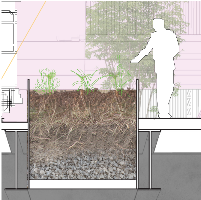
Raised educational beds in the demonstration garden, embedded in the bridges existing steel structure.
