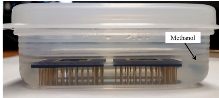
Figure 5.5: Chips stored in a container while immersed in methanol.
