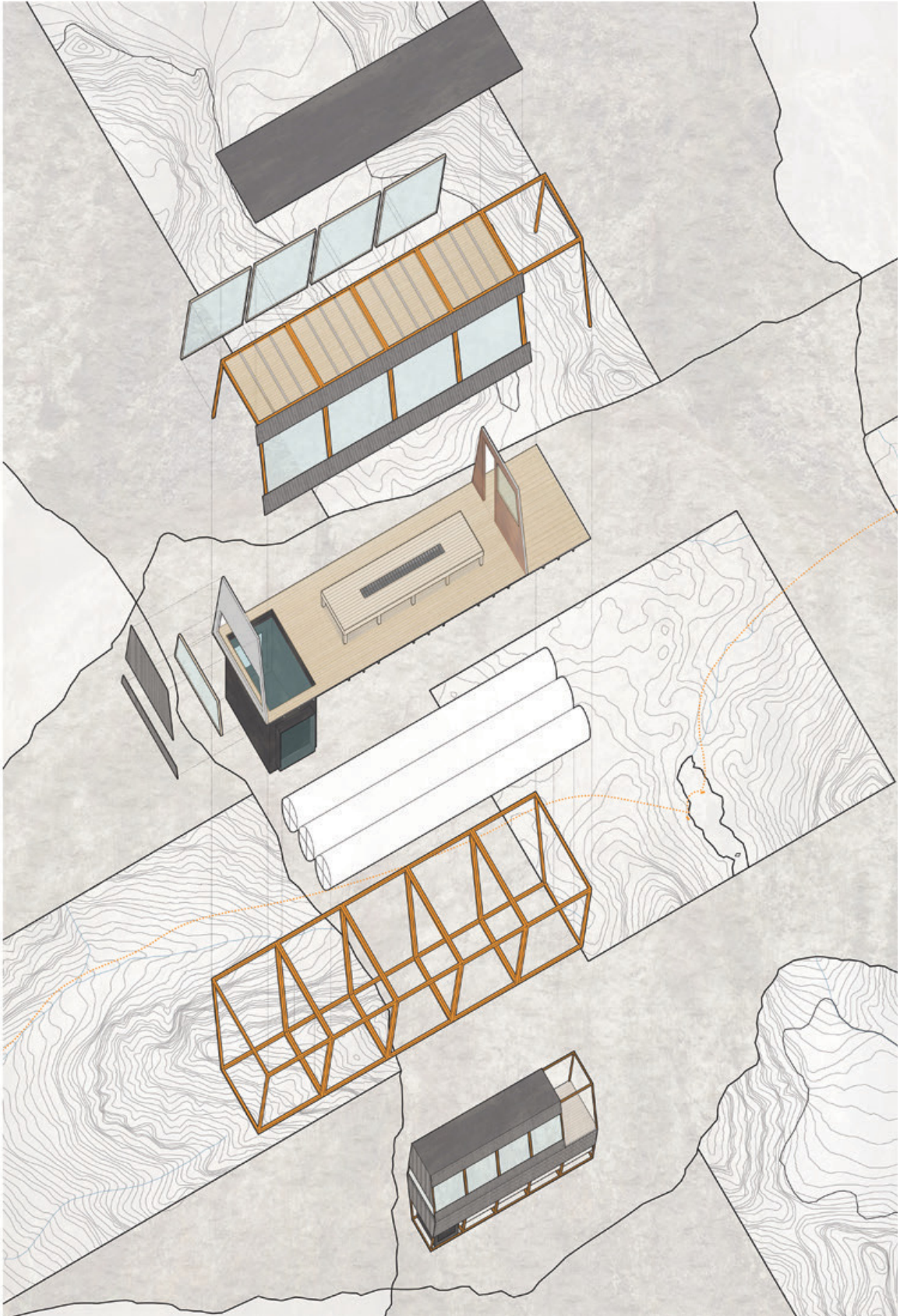
Figure 41. Exploded axo of floating sauna.
