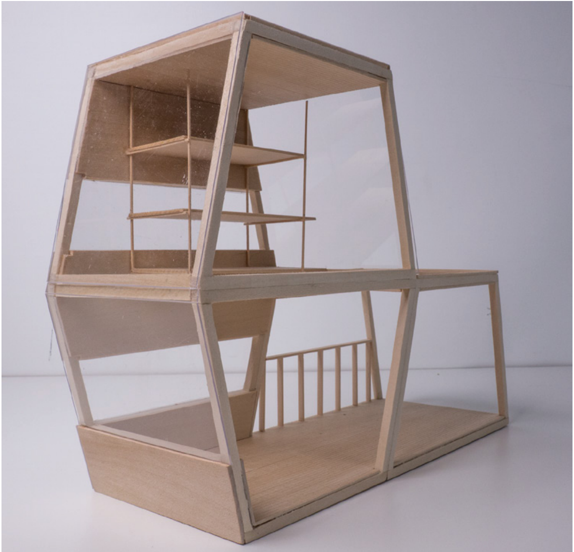
Figure 44. Model of shelter, showing the modular structures with different cladding options; from Patrick Spelliscy.
