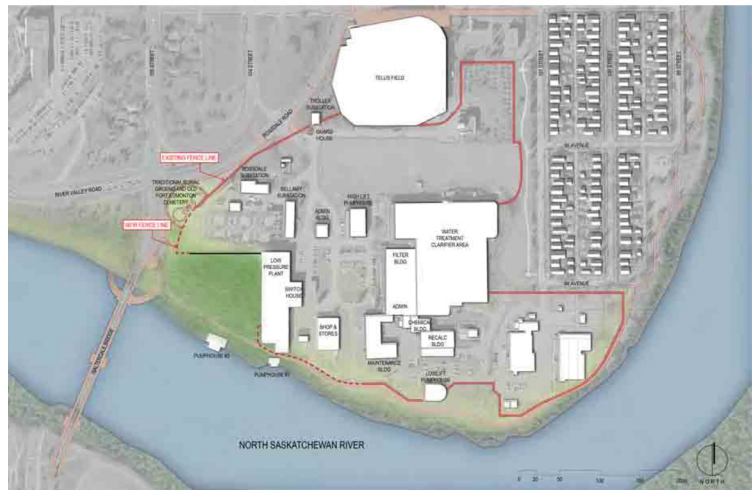
Current site plan, the red line represents the fence surrounding Epcor properties and the green shade represents the demolished building areas (Alberta Register of Historic Places 2016)
