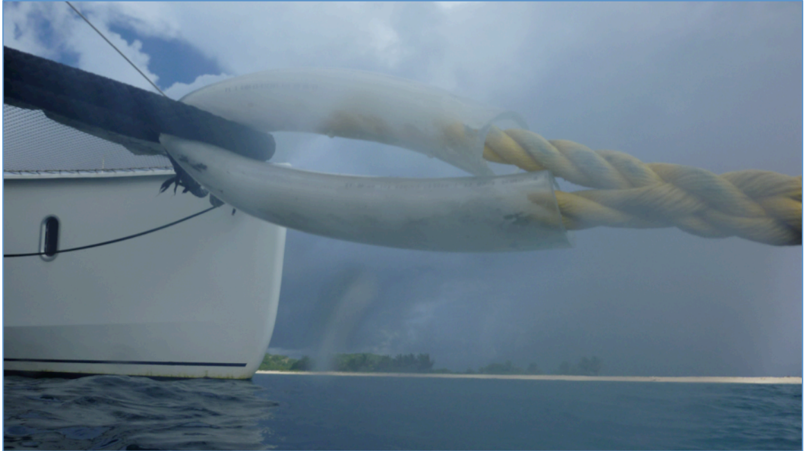
Figure 30. Image of the standard pick-up line with spliced rope loop reinforced with plastic piping to reduce abrasion from vessel lines (Reed, 2016).
