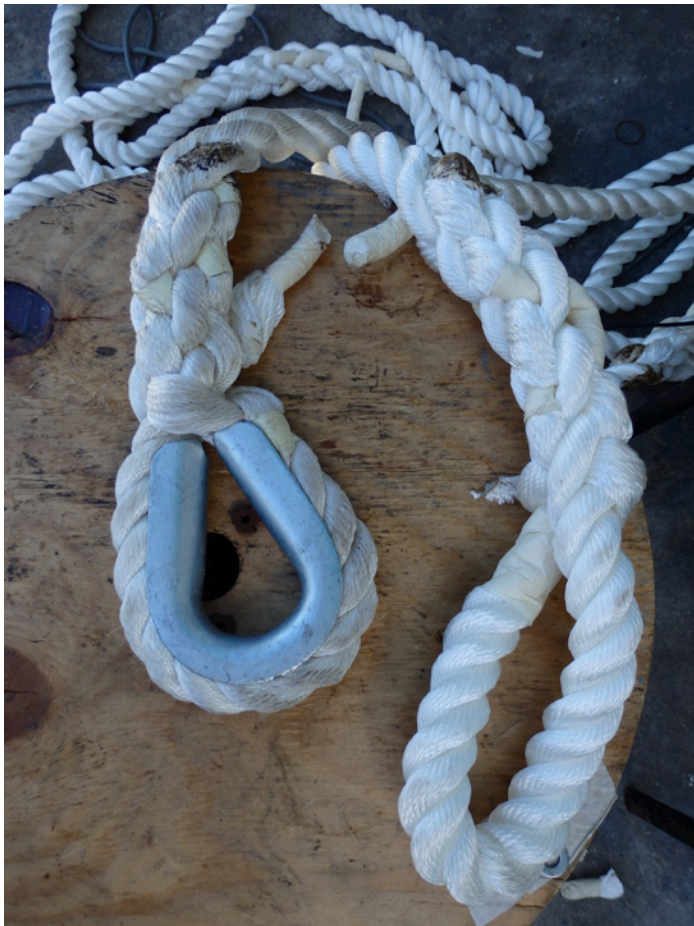
Figure 36. Image of a pickup line being made with spliced rope and a loop reinforced with steel, TCMP office, Union Island, SVG (Reed, 2016).
