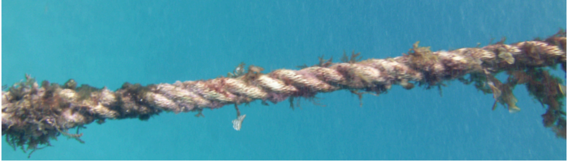
Figure 27. Image of downline with moderate fouling, TCMP (Reed, 2016).
