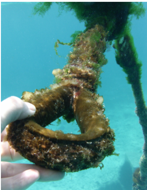
Figure 29. Image of the standard pick-up line with steel timble spliced into the looped rope to prevent abrasion, TCMP (Reed, 2016).
