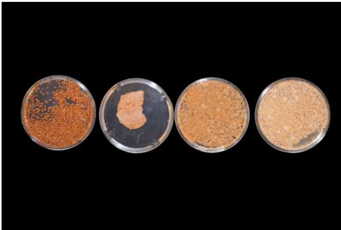
Figure 4.1. Samples of Camelina sativa seed, expelled cake, expelled meal, and expelled solvent extracted meal (SEM; in order of appearance from left to right), colour change is notable between the expelled meal and SEM
