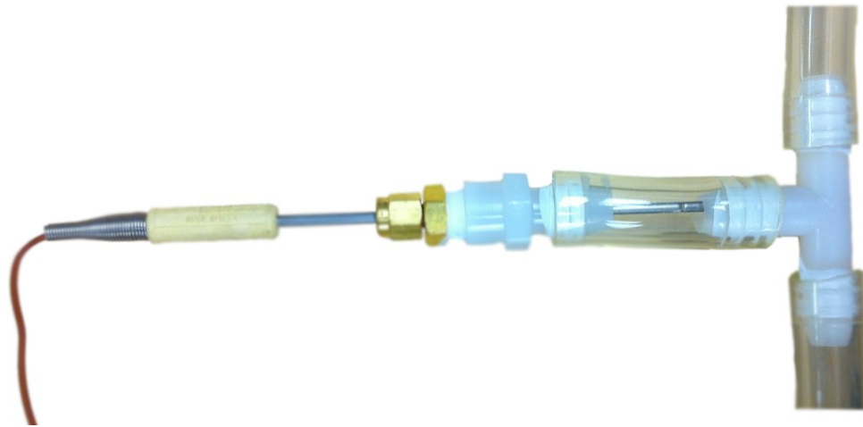
Fig. 5.6 – Image of K-type thermocouple and tee assembly
