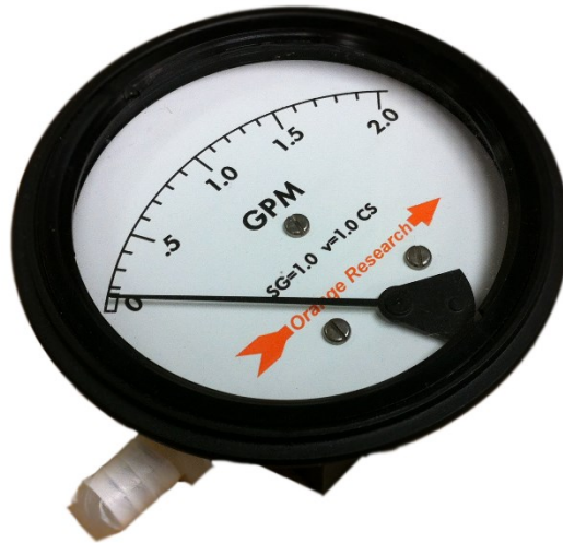
Fig. 5.4 – Image of mechanical flowmeter used in internal and external flow loops
