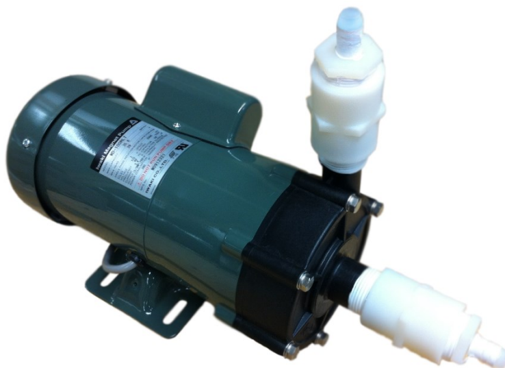
Fig. 5.3 – Image of centrifugal pump used in the internal flow loop
