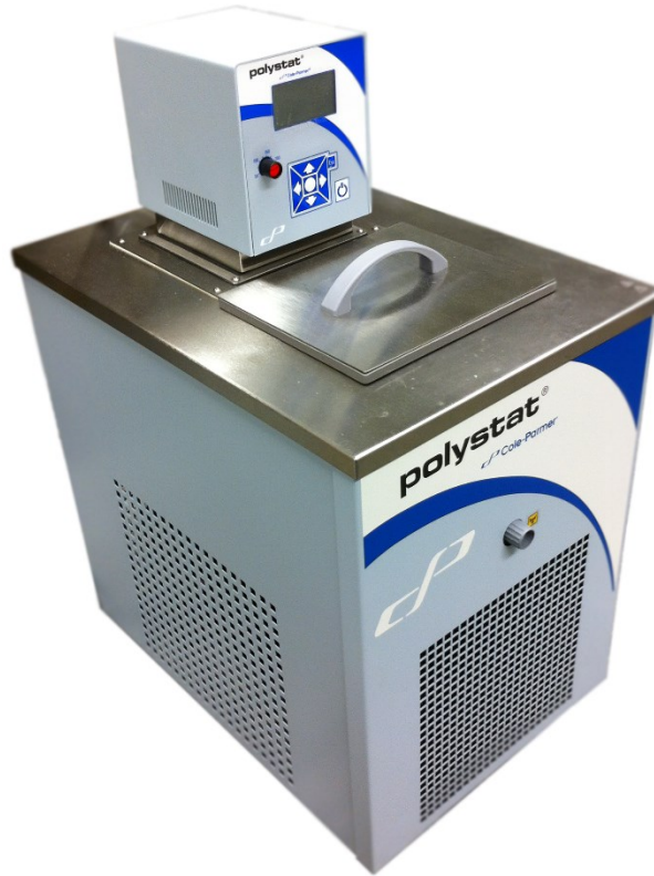
Fig. 5.5 – Image of recirculation chiller used in the external flow loop
