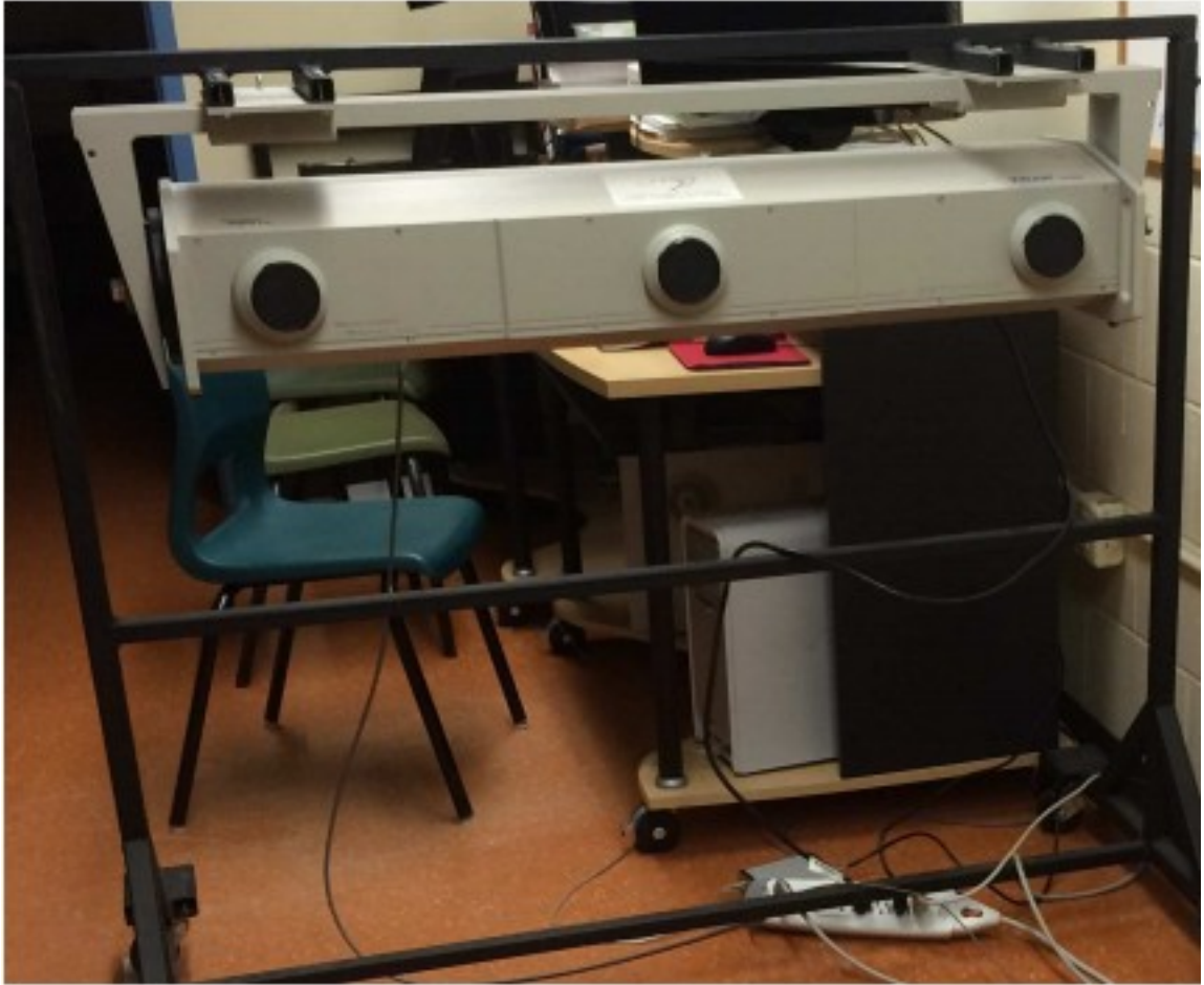
Figure 3-2: Optotrak 3020™ Motion Capture System. The Optotrak 3020™ 3D motion-capture system consisting of three infrared detecting cameras (Bishop & Westwood, 2016).
