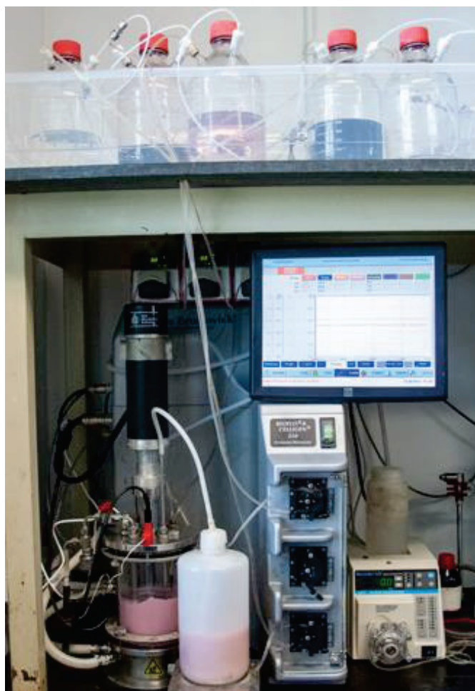
Figure 2.2 Continuously-stirring tank reactor
