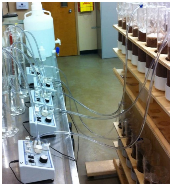
Figure 3.4 Leaching of 300 mL of 0.001 M CaCl 2 solution using pumps.
