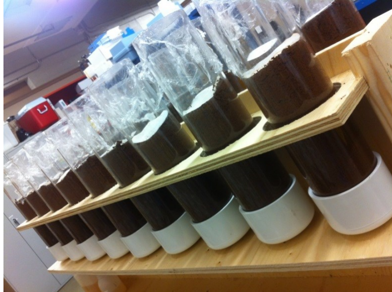
Figure 3.3 Picture showing columns filled with soil and biochar.
