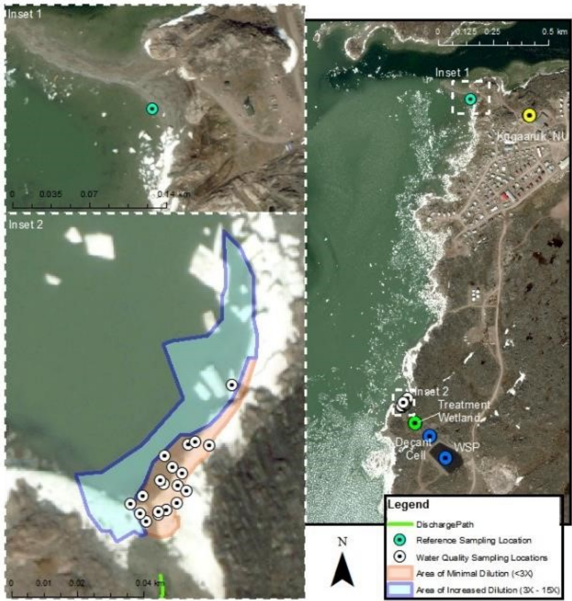
FIGURE 4.4. DELINEATION OF THE DILUTION ZONES AND WATER QUALITY SAMPLES IN KUGAARUK, NU.
