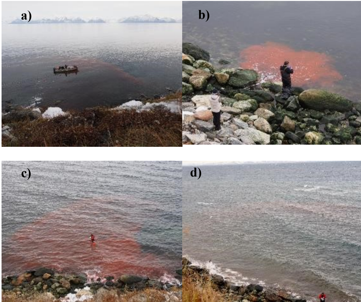
FIGURE 4.5. PHOTOGRAPHS OF THE RECEIVING ENVIRONMENT IN POND INLET, NU SHOWING THE: A) TRACER STUDY MONITORING FROM A BOAT ON SEPTEMBER 17, 2013; B) INITIAL MIXING OF THE DYE AT THE DISCHARGE LOCATION ON SEPTEMBER 12, 2013; C) NEAR-SHORE MONITORING OF THE DYE PLUME ON SEPTEMBER 15, 2013; AND D) LONG-RANGE TRANSPORT OF THE DYE ON SEPTEMBER 15, 2013.
