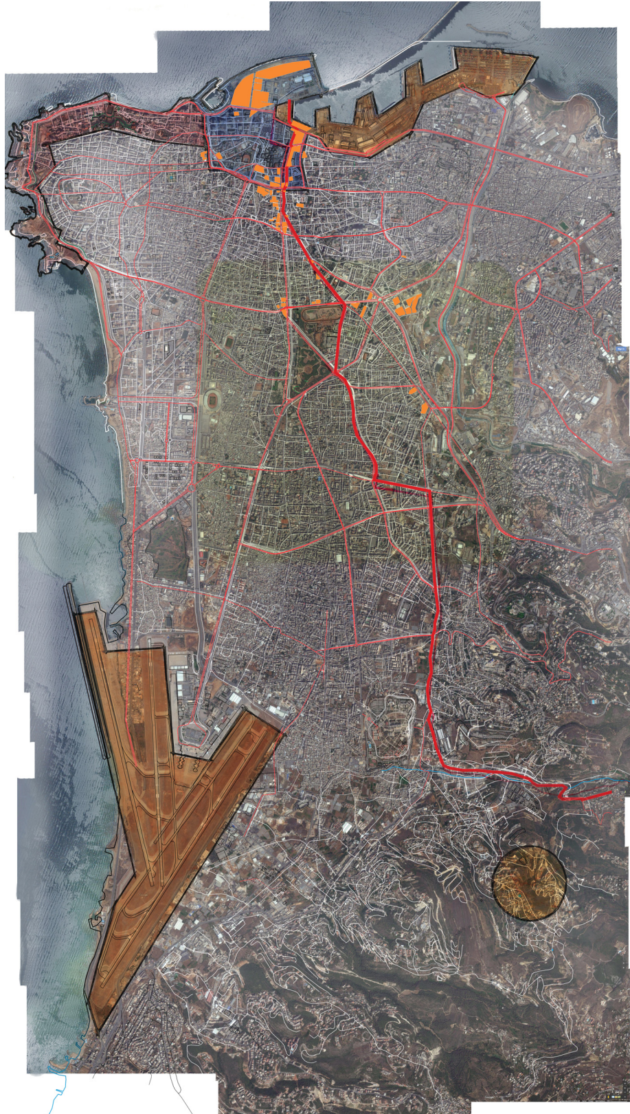
Map of Beirut showing potential tram lines (red) connecting the potential sites (orange), and the major points: port, airport, roadways(orange), BCD (blue), hotel district (pink), and city proper (green) (data from GoogleEarth 2016).
