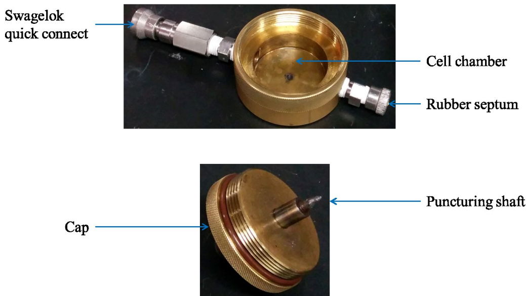
Figure 4.3. Picture of the gas extraction device designed for the extraction of gaseous and volatile components of Li-ion cells. Designed with the help of Simon Trussler, Physics & Atmospheric Science, Dalhousie University (2014). The outer diameter of the chamber was 7.5 cm.
