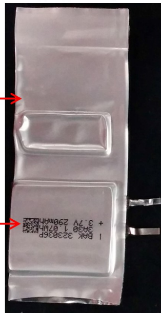
Figure A1. Picture of NMC/graphite and LCO/graphite pouch cells used throughout the work presented in this thesis. NMC(442)/graphite, NMC(111)/graphite and LCO/Si:graphite pouch cells have the same format.
