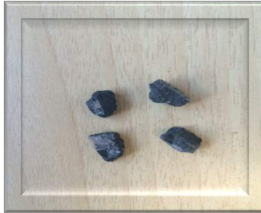
Figure 6.8 Concrete specimens for MIP test
