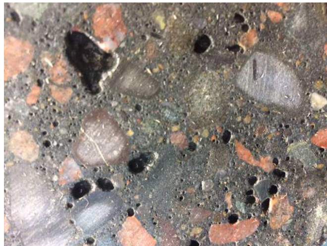
Figure 2.9 Influence of poor compaction and vibration on concrete matrix made with blended cement
