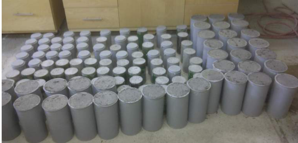
Figure 6.1 Concrete cylinders tested in the project
