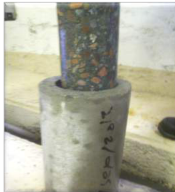
Figure 6.2 Extracting of concrete cores from larger cylinders
