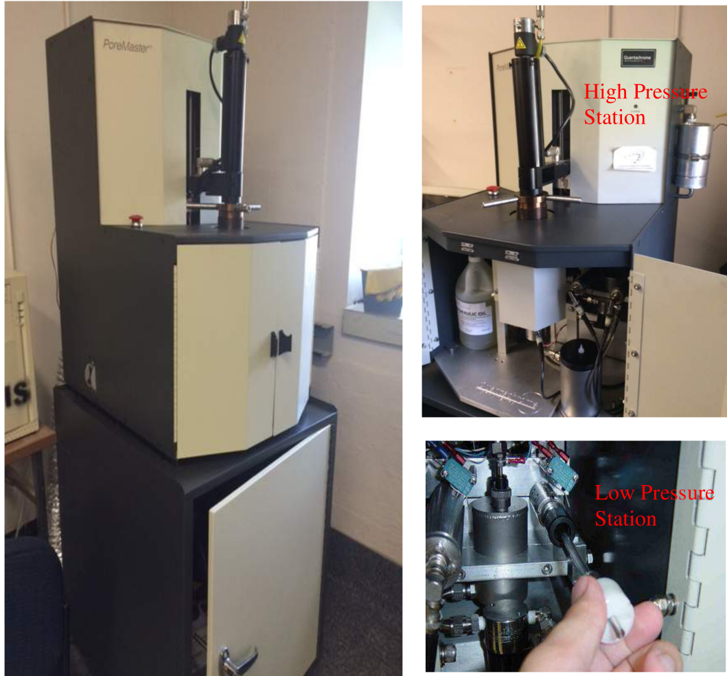
Figure 6.9 Quantachrome Poremaster - 33 apparatus (MIP) test
