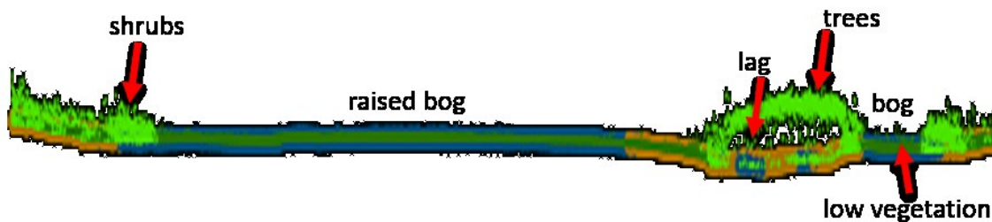
Figure 2.4: Profile of transitioning wetland classes, with terrain and vegetation height extracted from lidar points.
