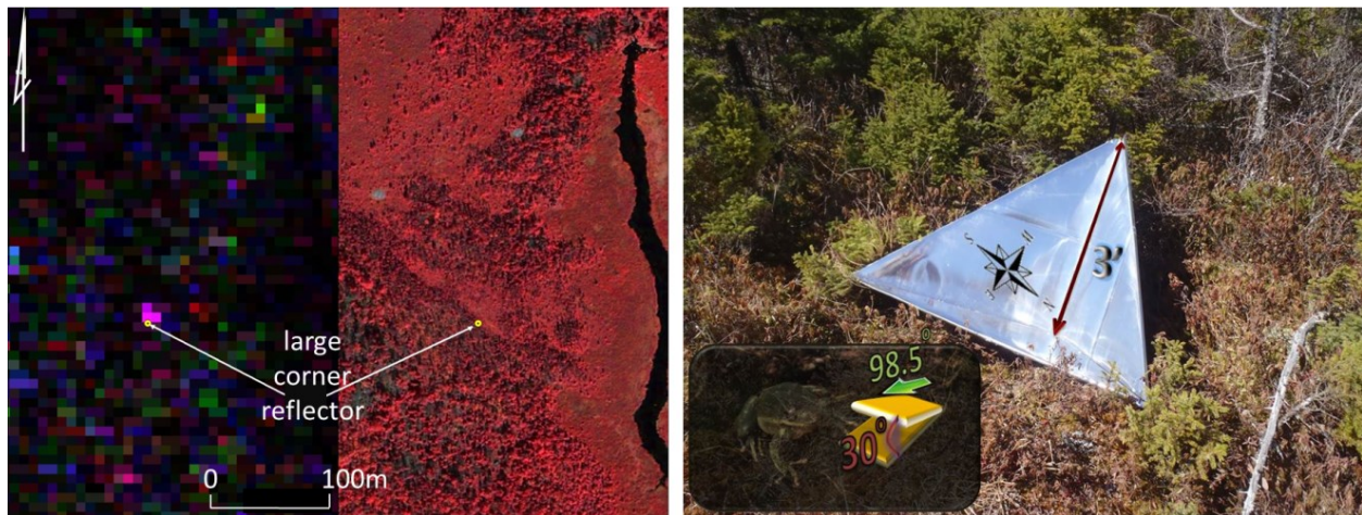
Figure 3.10: A radar reflector was set up at an open wetland transitioning into treed to assess positional accuracy.
