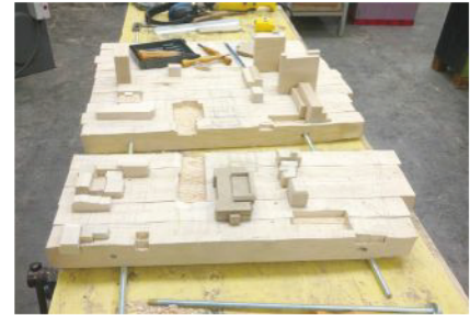
Threaded rod and wood connections allowed for the model to be disassembled to work on.
