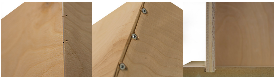
Figure 58. 1:10 material testing with 3 types of connections. Left) Glue and nail. Middle) Screwed in fasteners. 3) Wood joint connectors.
