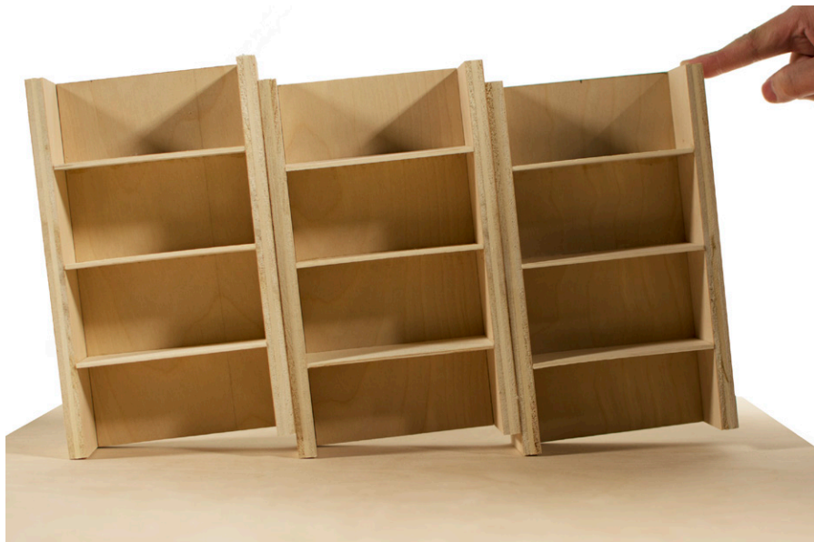
Figure 50. Each module reacts in isolation when put under lateral stress.
