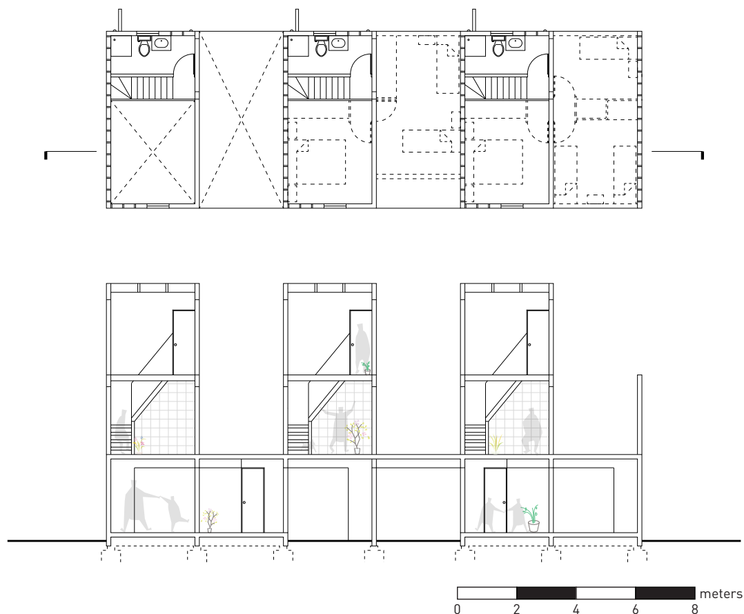
Figure 88. Floor plan and sections of the modular housing units created for incremental design by Elemental, data from Aravena, Elemental: A do Tank.
