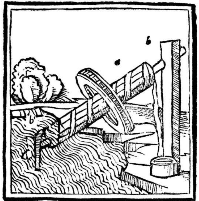
Fig. 10. The water screw, Book X. (Collection Woodward Library, University of British Columbia)
