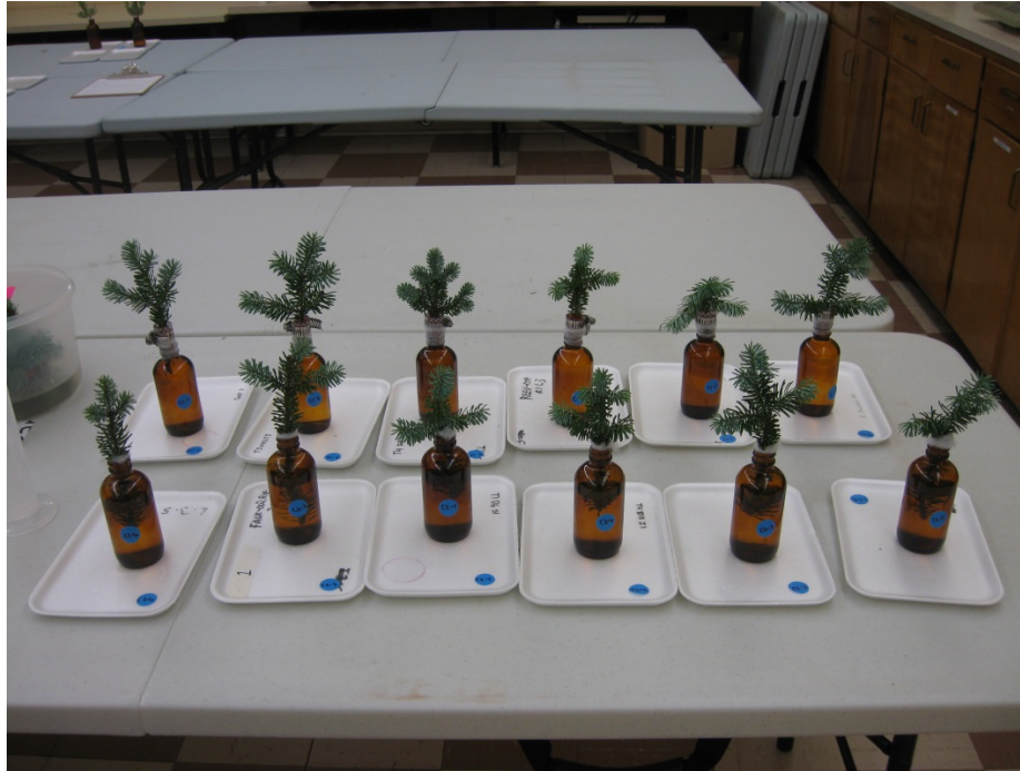
Figure 8.2 Setup of the control branches. Branches in the back row were fitted with a section of tubing meant to simulate the possible restricting effect of the root pressure system on water uptake. Branches in the front row were not subjected to this restriction.
