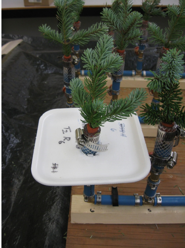
Figure 8.6. A section was cut from a foam tray to fit around the pipe containing the pressure-treated branch. The tray was fitted under the branch, and the section was replaced to secure the tray. The tray was transferred from one branch to the next during the finger-run test and needle collection.
