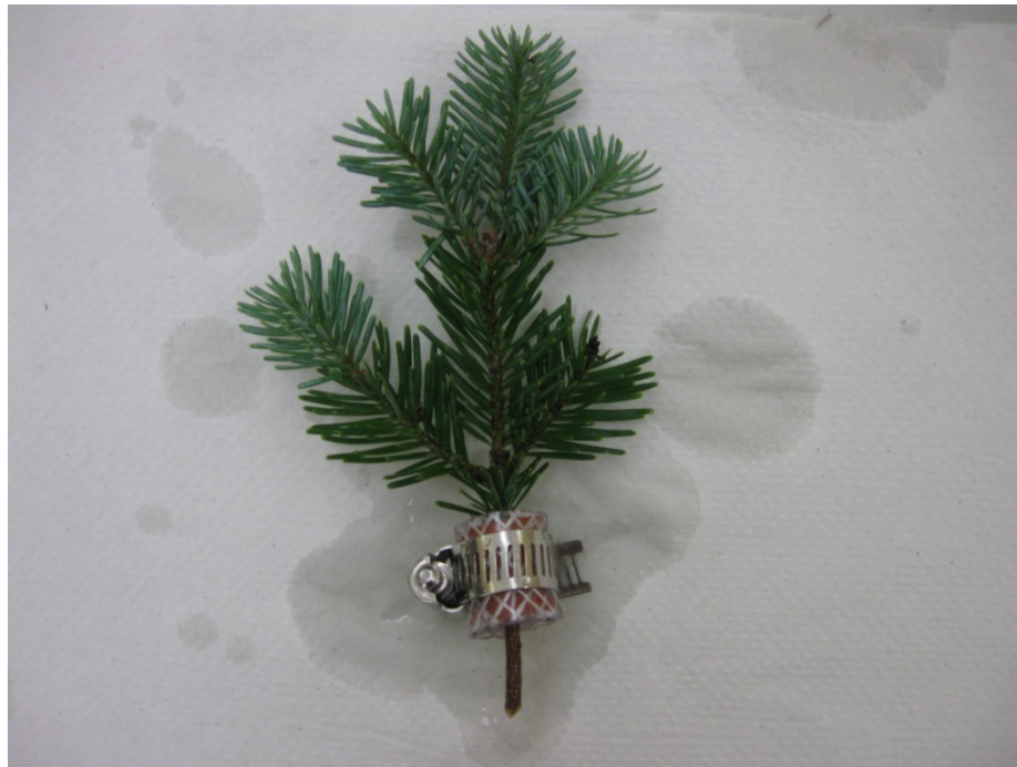
Figure 8.1 Six control branches were fitted with a short section of 3/4" clear braided vinyl tubing to simulate the possible restricting effect of the root pressure system.
