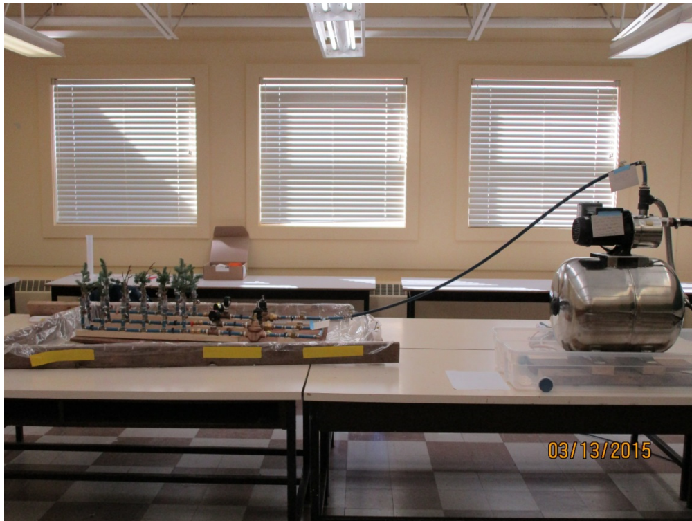
Figure 8.5 Setup of the root pressure system. Water was distributed to the manifolds (left) by a 16-gallon shallow well jet pump (right).
