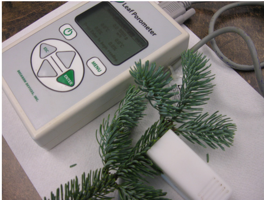
Figure 3.2 Taking a conductance reading from attached needles.
