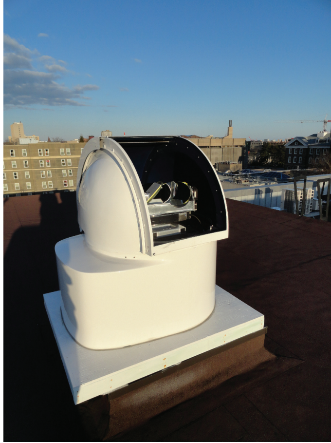
Figure 4.4: Image of the CST operating within the protective RoboDome on the roof of the DAO.
