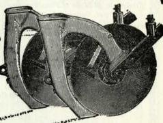
O SOW properly, all seed must be put in at even depth across the drill. By so doing, the crop all sprouts at the same time, and ripens evenly later. This advantageous yield is insured by a strong I-beam, which holds up the centre drills against sagging. Accurate seeding is essential to right sowing also. Unlike many seeders, the Cockshutt feed device is protected from jolting and derangement by the wheels. You still have accurate distribution after years
