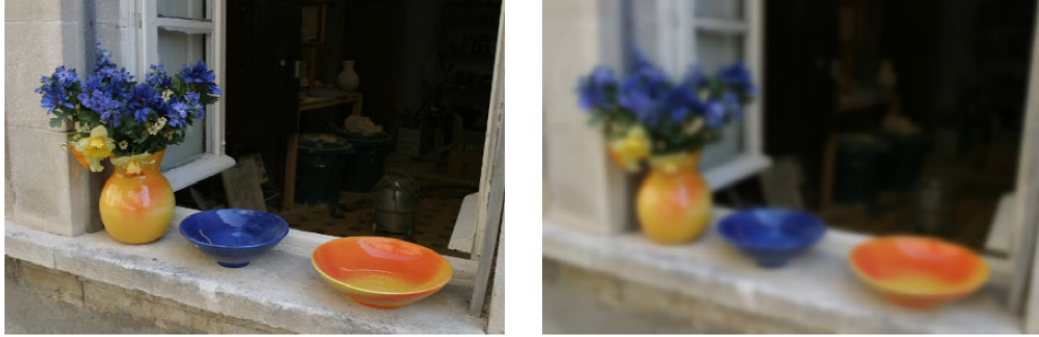
Figure 2.12 Source image (left) applies Gaussian filter to show blurry effects [25]
