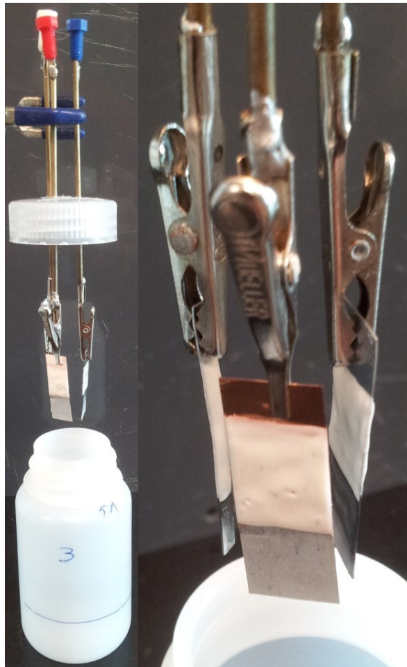
Figure 4-1: Experimental apparatus for the foil experiments. The container is a 125 mL Nalgene bottle. The rods are brass and are soldered to Ni plated alligator clips (some with teeth, others flat). Foils of particular widths and heights are cut and partially covered in water resistant epoxy such that 1.00 \pm 0.05 cm remained uncovered from epoxy to bottom edge.
