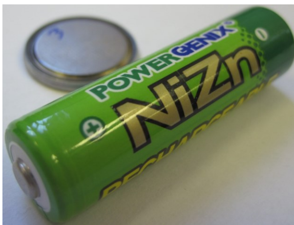
Figure 2-16: PowerGenix AA cell tested in the same manner as the coin cells (also shown). These cells are rated to provide between 1350 and 1500 mAh. No expected cycle life is reported on the PowerGenix website.
