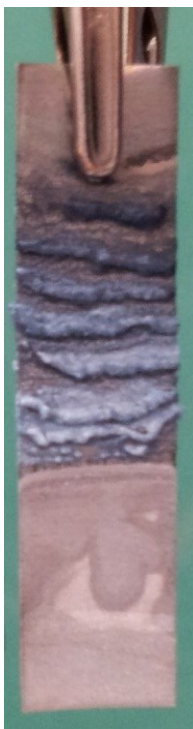
Figure 4-4: Demonstration of electrolyte wicking up conducting surfaces. This is a long Zn foil electrode that was dipped in 3.2 M KOH, saturated with ZnO and cycled.
