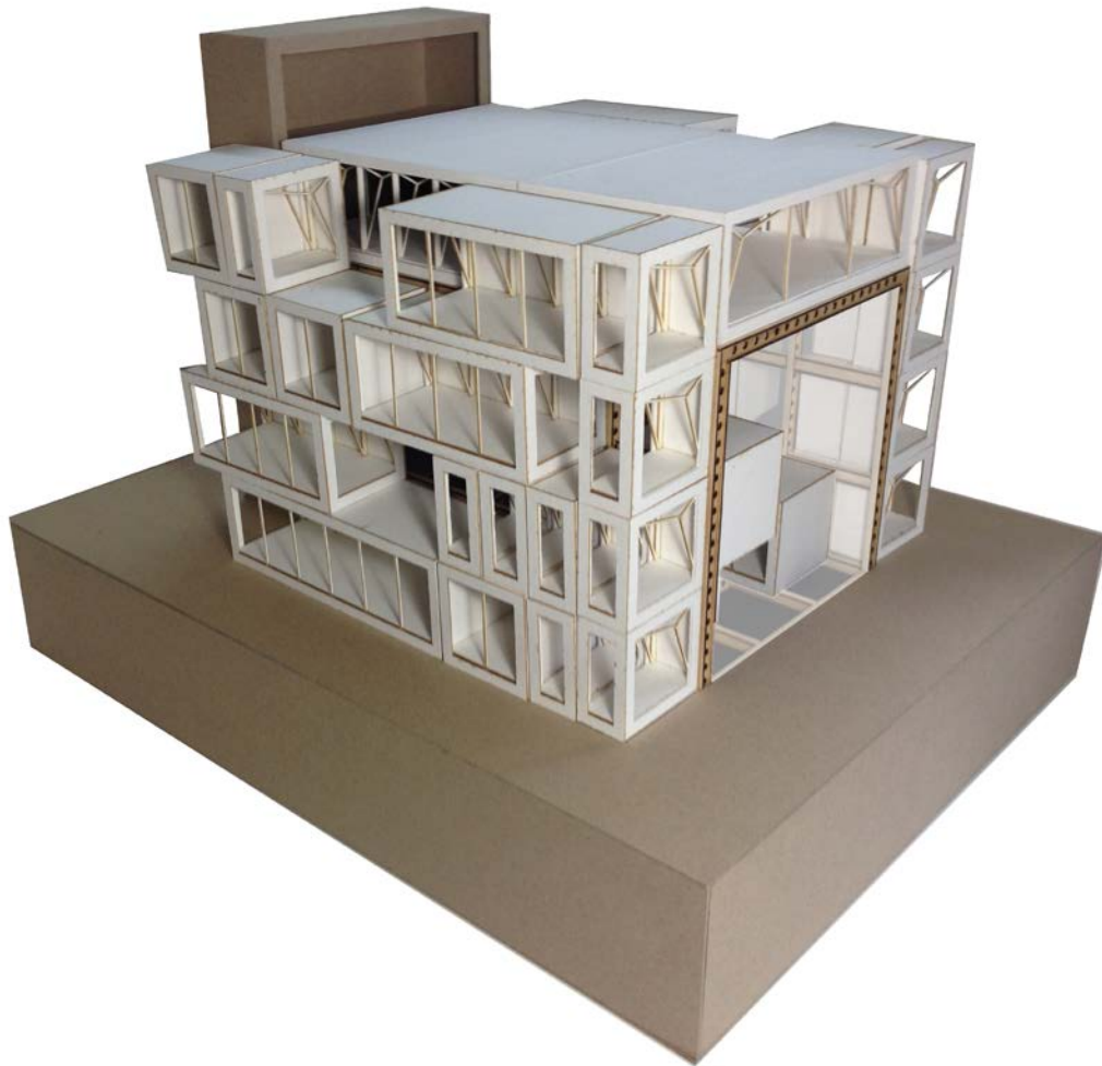
Image 46: Physical model of program modules showing one possible aggregation of the modules on the support manifold.
