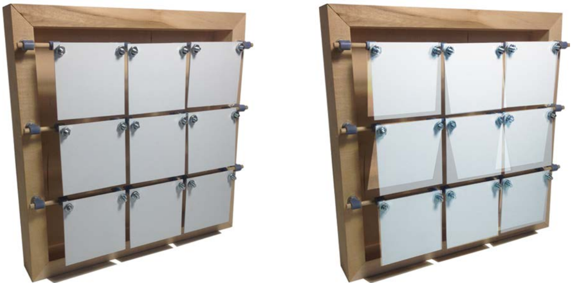
Image 65: Environmental-responsive, simple movement panel study, demonstrating a wind-actuated facade.
