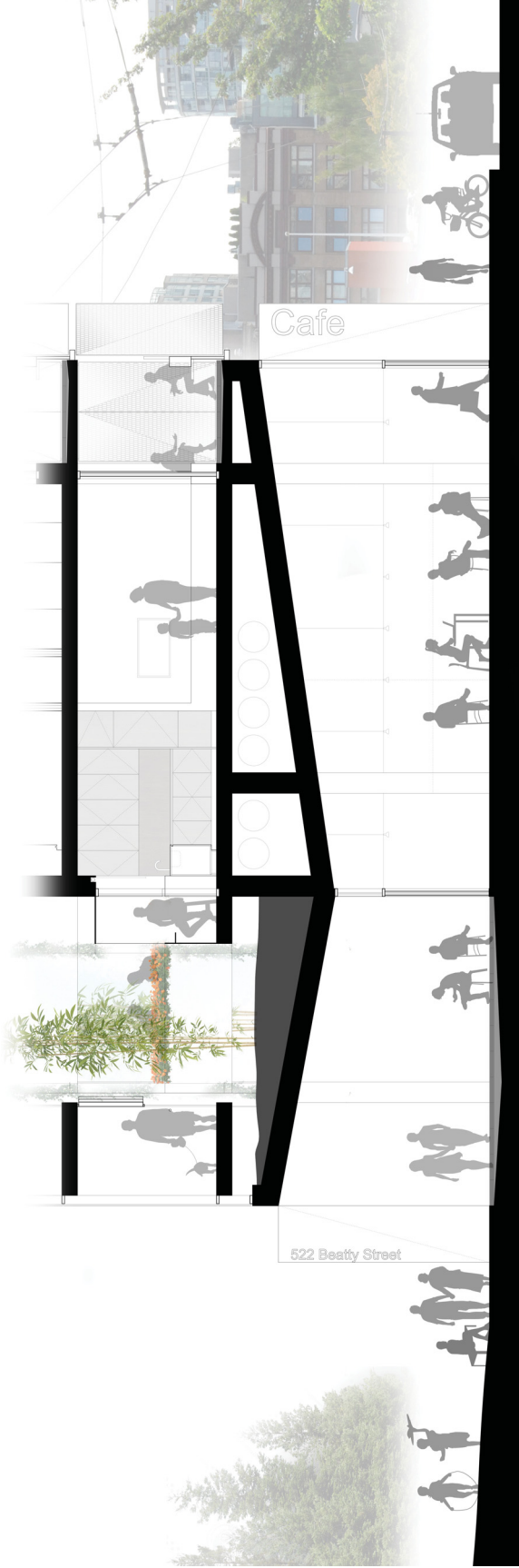
Section through one floor of the atrium, units, and balcony highlighting the architectural features mediating the boundary space between unit and circulation and unit and city. 1:80
