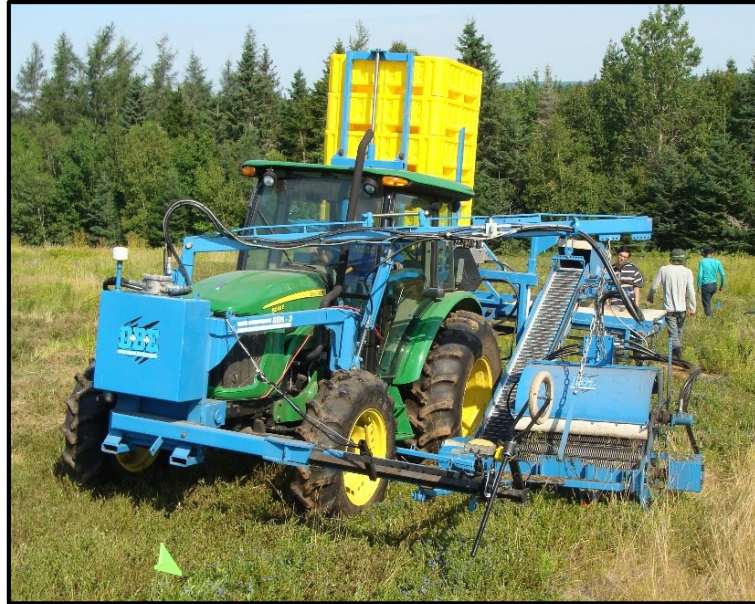
Figure 3-3: Single head wild blueberry harvester mounted on a John Deere tractor.
