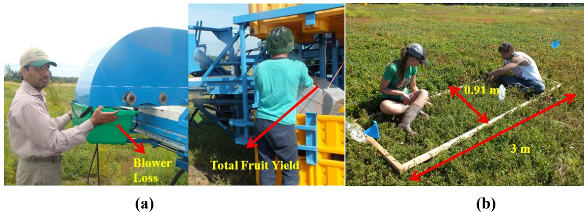
Figure 5-1: (a) Manual collection of fruit losses through the blower and total fruit yield and (b) Collection of fruit losses on the ground and un-harvested berries on the plants from the harvested plot.
