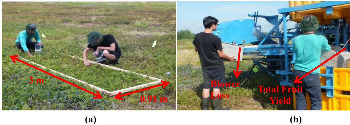
Figure 3-4: (a) Manual collection of loss on the ground and un-harvested berries on the plants; (b) Collection of fruit losses through the blower and total fruit yield from the harvested plot.
