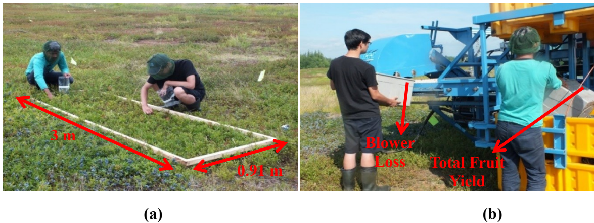
Figure 4-2: (a) Manual collection of loss on the ground and un-harvested berries on the plants; (b) Collection of fruit losses through the blower and total fruit yield from the harvested plot.
