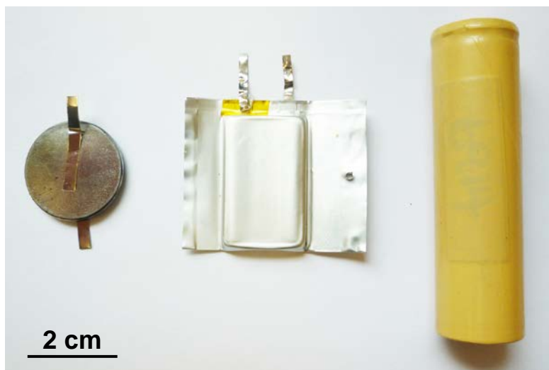
Figure 1.9: Three common lithium ion cell designs. From left to right: a coin cell, a flat-wound pouch cell, and a cylindrically wound cell.
