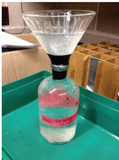
Figure 2.3: 500 ml sample bottle used to collect rainwater over the course of this study. Funnel diameter is \sim 135 mm.
