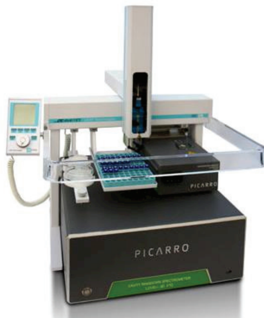
Figure 2.7: Picarro L2301-i WS-CRDS isotopic water analyzer used in this study.
