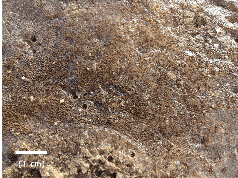
Figure 1.4: A photograph of the surface of a sediment-laden ice block, taken on February 23, 2012, shows that they are primarily comprised of ice, sediment and air. Small scale surface roughness is also apparent.
