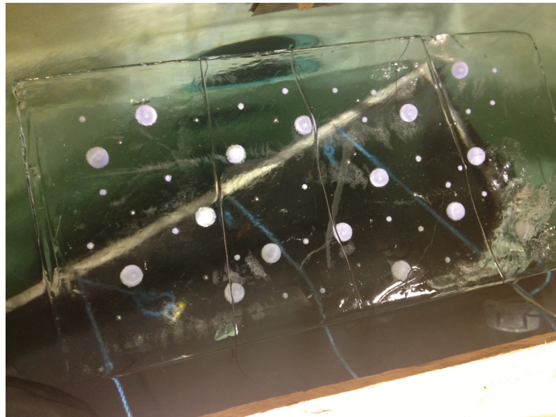
Figure 3.5: BLK3 (see Table 3.2) contains a mixture of different scattering obstacles encased in ice. Small tungsten-carbide spheres have been used to simulate sediment inclusions and polypropylene shells of different sizes have been used to simulate air cavities.
