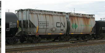
CN 399000 Articulated Covered Hopper. Photograph by Dan Dell'Unto, 2008, from Canadian Freight Railcar Gallery.
