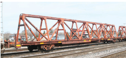
CN 54989 Turnout Panel Flatcar. Photograph by David Graham, 2010, from Canadian Freight Railcar Gallery.
