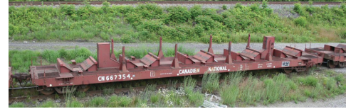
CN 667354 62' Coil Steel Flatcar. Photograph by Chris vanderHeide, 2008, from Canadian Freight Railcar Gallery.
