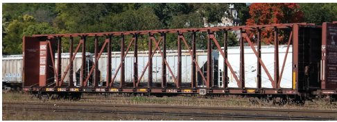
CNIS 623163 Centrebeam Flatcar. Photograph by Bernie Goodman, 2014, from Canadian Freight Railcar Gallery.
