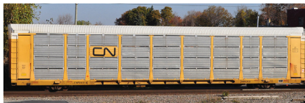
CN 704518 Enclosed Trilevel Autorack. Photograph by Pierre Lacombe, 2013, from Canadian Freight Railcar Gallery.
