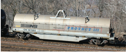
CN 187002 Covered Coil Steel Car. Photograph by David Graham, 2006, from Canadian Freight Railcar Gallery.
