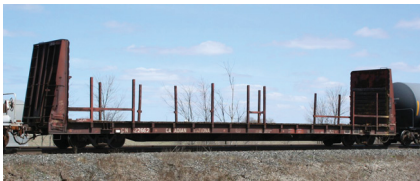
CN 622662 66' Bulkhead Flatcar. Photograph by Chris vanderHeide, 2013, from Canadian Freight Railcar Gallery.
