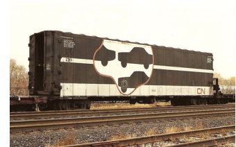
CN 9504 Double Deck Automobile Transporter. Photograph by Alex Simins, 1991, from Canadian Freight Railcar Gallery.
