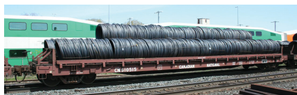
CN 610515 56' Wire Flatcar. Photograph by Chris VanderHeide, 2007, from Canadian Freight Railcar Gallery.
