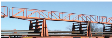
CN 46504 Welded Rail Flatcar. Photograph by David Graham, 2008, from Canadian Freight Railcar Gallery.
