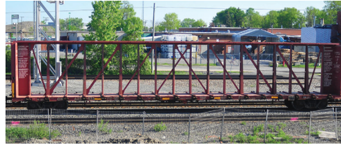
CN 625533 73' Centre-beam Bulkhead Flatcar. Photograph by Pierre Lacombe, 2013, from Canadian Freight Railcar Gallery.
