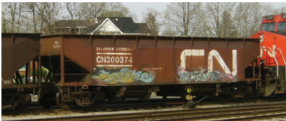
CN 300374 Offset-Side Longitudinal Hopper. Photograph by Chris vanderHeide, 2004, from Canadian Freight Railcar Gallery.
