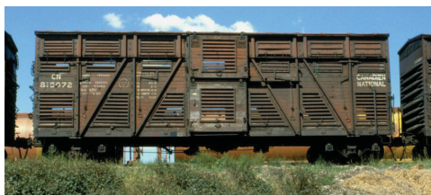
CN 815072 40' Stock Car. Photograph by Andy J. Broscoe, 1981, from Canadian Freight Railcar Gallery.
