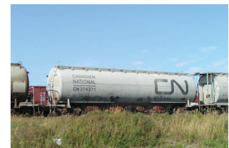
CN 374271 Pressure Unloading Covered Hopper. Photograph by Marc-A. Hudon, 2004, from Canadian Freight Railcar Gallery.
