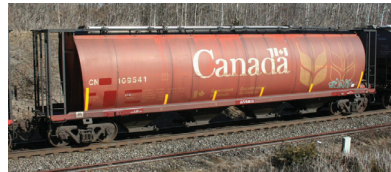
CN 109541 Cylindrical Covered Hopper. Photograph by Chris vanderHeide, 2009, from Canadian Freight Railcar Gallery.
