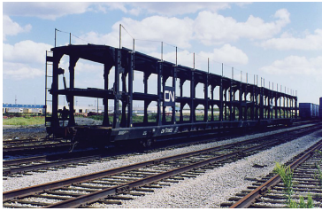
The three story automobile car was used as a starting point for the energy car. The CN 700652 Open Trilevel Autorack. Photograph by Brian Switzer, 1998, from Canadian Freight Railcar Gallery.
