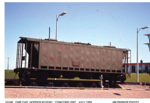
CN 135228 Slab-Side Covered Hopper. Photograph by Jim Parker, 1965, from Canadian Freight Railcar Gallery.
