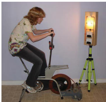
A girl using her stationary bike to power a lamp. Photograph by Wingsinger, 2012, from "Turn an exercise bike into an energy bike".
