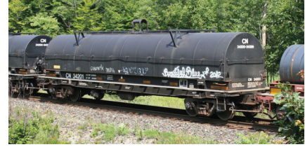
CN 34201 Coil Steel Car. Photograph by Chris vanderHeide, 2014, from Canadian Freight Railcar Gallery.
