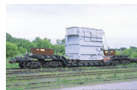
CN 675001 Depressed Centre Flatcar. Photograph by Brian Switzer, 2000, from Canadian Freight Railcar Gallery.
