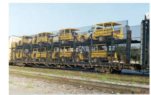
CN 710657 Open Bilevel Autorack. Photograph by Bernie Goodman, 1998, from Canadian Freight Railcar Gallery.
