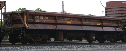
CN 56120 Side-Dump Ballast Gondola. Photograph by Ed Cooke, 2010, from Canadian Freight Railcar Gallery.
