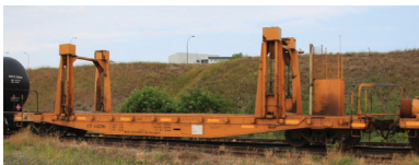
CN 44296 Welded Rail Unloading Car. Photograph by Colin Restorick, 2009, from Canadian Freight Railcar Gallery.
