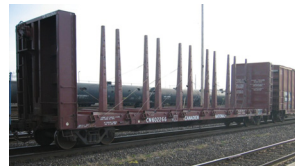
CN 602266 51' Centre-Post Bulkhead Flatcar. Photograph by David Graham, 2004, from Canadian Freight Railcar Gallery.
