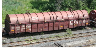
CN 188410 52' Covered Gondola. Photograph by Chris vanderHeide, 2012, from Canadian Freight Railcar Gallery.
