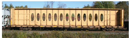
CNA 623052 Centre-beam Flatcar. Photograph by Chris VanderHeide, 2008, from Canadian Freight Railcar Gallery.
