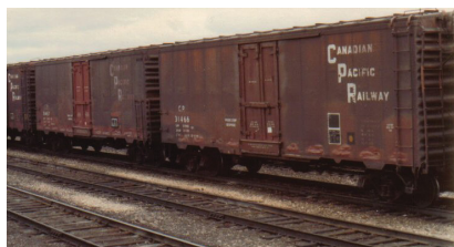
CP 31466 40' Woodchip Boxcar. Photograph by Eric Gagnon, 1981, from Canadian Freight Railcar Gallery.
