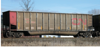
CNA 192022 Rotary Dump Coal Gondola. Photograph by William Henderson, 2013, from Canadian Freight Railcar Gallery.
