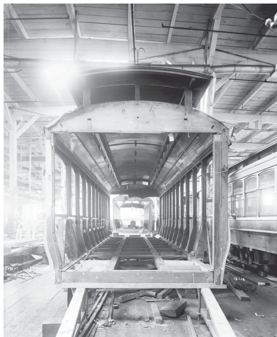
Partially constructed B.C. Electric Railway Company streetcar, 1914. Major James Skitt Matthews. From City of Vancouver Archives, AM54-S4-: LGN 914.
