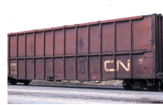
CN 873097 52' Woodchip Gondola. Photograph by William Henderson, 1977, from Canadian Freight Railcar Gallery.
