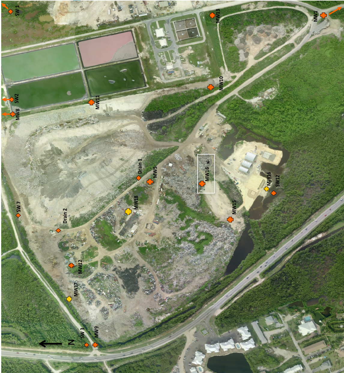
Figure 2.1. Map of DEH's GTLF monitoring sites. Figure shows map of monitoring sites used by DEH for water quality testing at GTLF. Surface water is analyzed at SW sites [surface water]. Groundwater is analyzed at MW sites [monitoring well]. Note that *MW16, should say MW14. (Source: Johnson, 2014).
