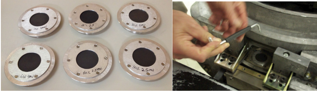
Figure 3.3: Left: Manufactured carbon targets in their aluminum holders. Right: Low-Z target being installed in the carousel of a Varian 2100 C linac.
