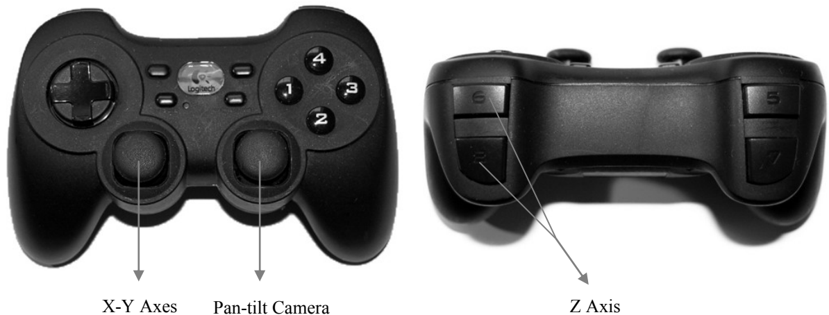
Figure 5.5. The model of the gamepad used in this thesis, Logitech Rumblepad 2, has two analog sticks. One of them is used to move the WireCam in X-Y direction and another one is for controlling the pan-tilt camera. The wire-suspended system is moved in Z direction using the right shoulder button pair.
