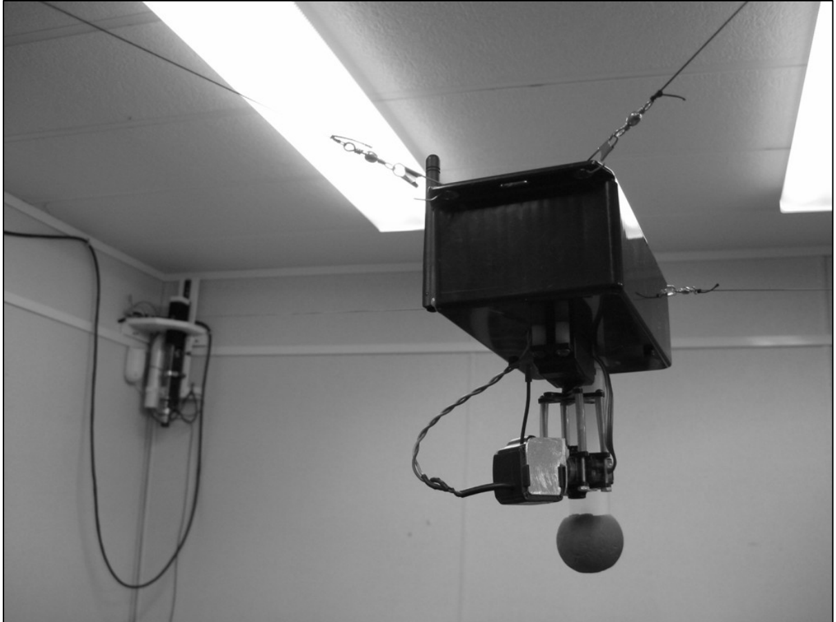
Figure 5.13. The actual WireCam with the Flying-Base in the middle and one of the winches in the left background
