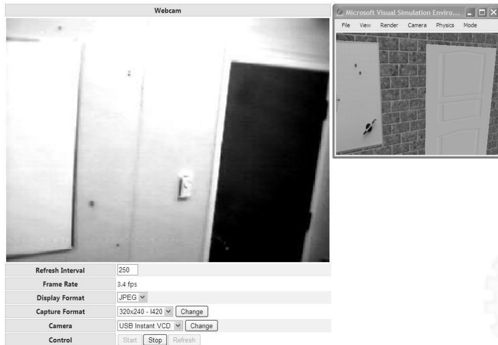
Figure 5.16. A screenshot of Operator PC during remote control of the WireCam
