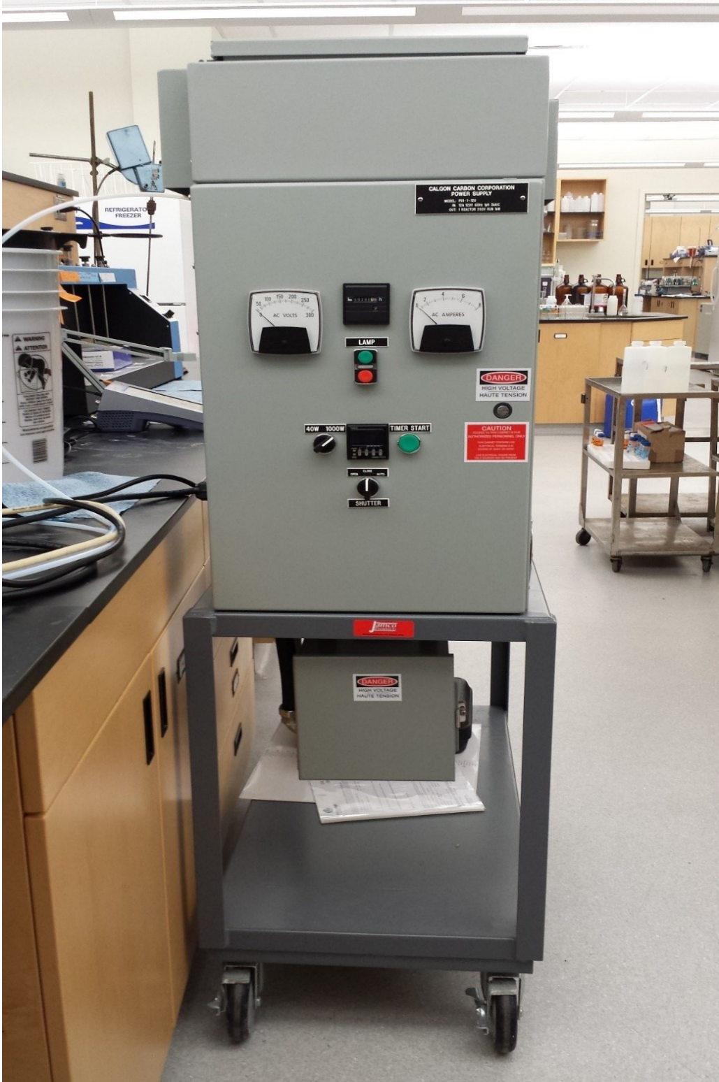
Figure 3-4 Bench-scale Calgon Carbon collimated beam unit
