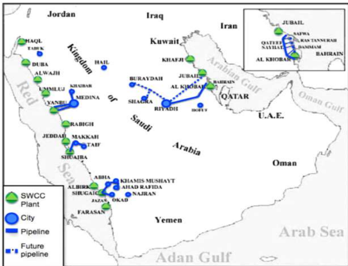
Figure 5-2 Desalination plants and pipelines controlled by SWCC (Source: SWCC, 2010)
