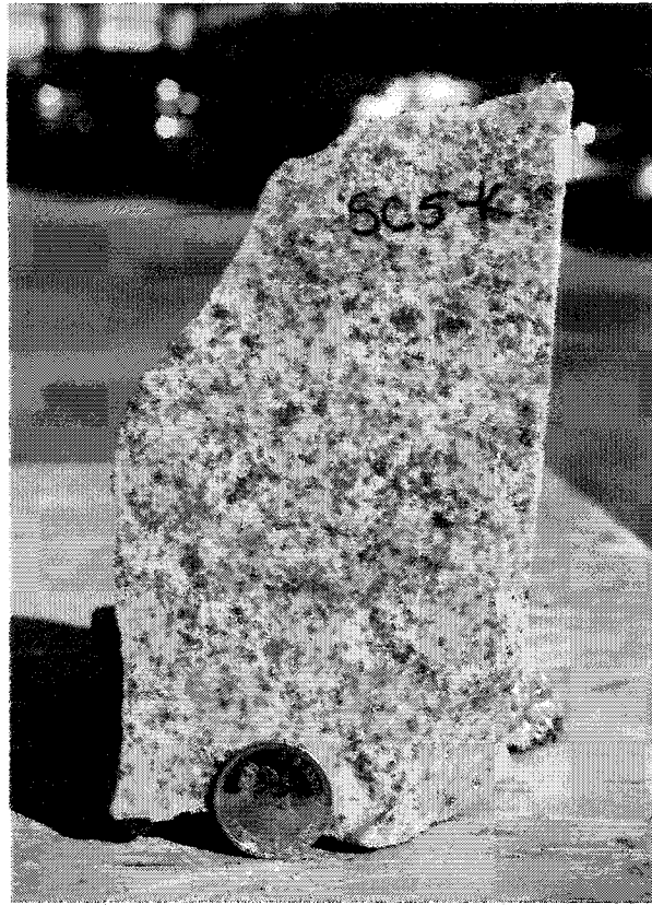
Fig. 2.10: Greisenised leucomonzogranite (SC-5-K) from the Keddy prospect. The rock is fine-grained and contains a high modal proportion of white mica. This sample is slightly hematized. Diameter of coin: 23 mm.
